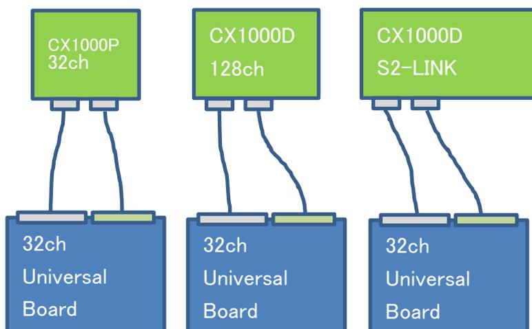
Case 3) For larger circuit (i.e. larger area) is required for device testing, larger universal board such as 128ch or 256ch universal board is available for smaller system, such as CX1000P.
