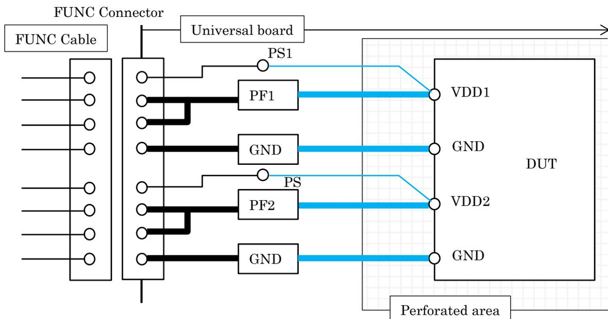
**Fig. 5 Power sense and force position**
