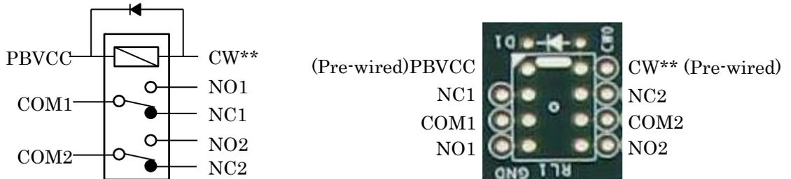
For mechanical relay signals, paired GND to relay pins do not exist.
